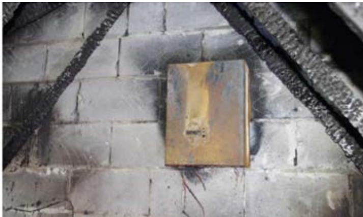
Photo: BRE Fire and Solar PV systems-Investigations and Evidence showing Inverter fire (Part of 3-year study by BRE, published July 2017 by BEIS)
