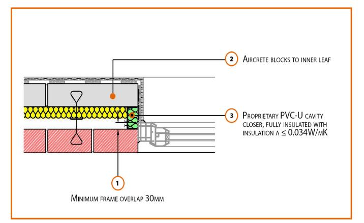
External Masonry Cavity Wall
