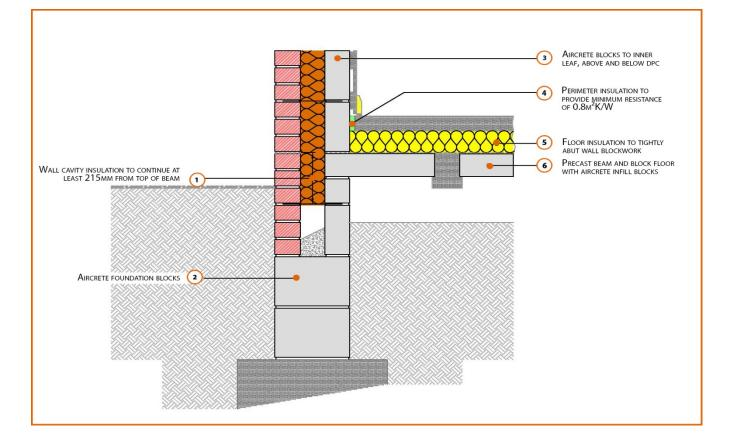
External Masonry Cavity Wall
