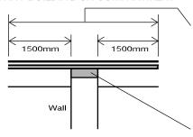
Roof covering over this distance to be designated AA, AB or AC on deck of material of limited combustibility. Roof covering and deck could be composite structure. E.g. profiled steel cladding.
