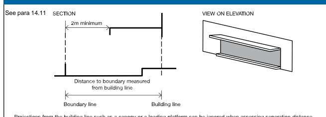
Projections from the building line such as a canopy or a loading platform can be ignored when assessing separation distance. This would not apply to an enclosed loading bay, for example if the illustration had shown side walls beneath the canopy.
