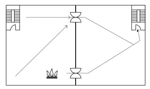
Storey divided into two refuges by compartment wall (stairways not provided with wheelchair space).
