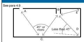
Alternative routes are available from C because angle ACB is 45° or more and therefore CA or CB (whichever is the less) should be no more than the maximum distance for travel given for alternative routes.
