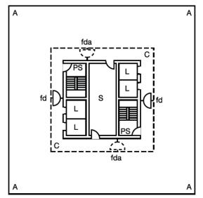
Note: The doors at both ends of the area marked 'S' should be self-closing fire doors unless the area is sub-divided such that any fire in that area will not be able to prejudice both sections of corridor at the sam time. If that area is a lift lobby, doors should be provide as shown in Figure 8 in BS 5588: Part 11: 1997.
