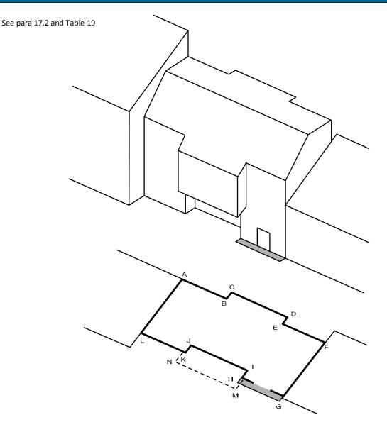
Plan of building AFGL where AL and FG are walls in common with other buildings.
