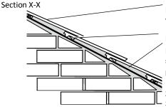
Roof covering to be designated AA, AB or AC for at least 1500mm either side of wall
